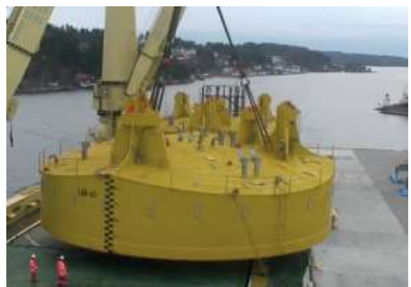
Jack-up rig leg "spud can" removed for maintenance
