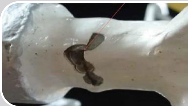
Event 1 – Crack in small bore piping
