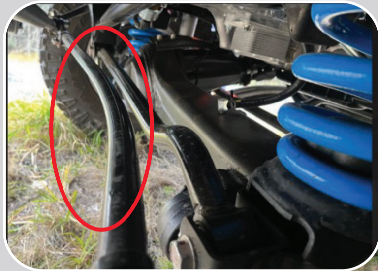
Bent steering drag link following impact.
