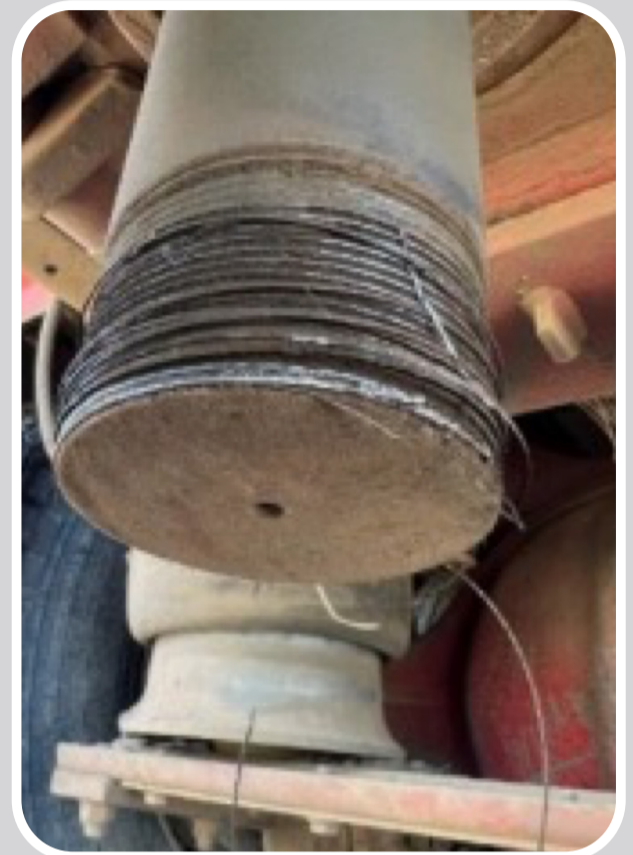
Thread wear on main nut locking pin of flying saucer hitch assembly.
