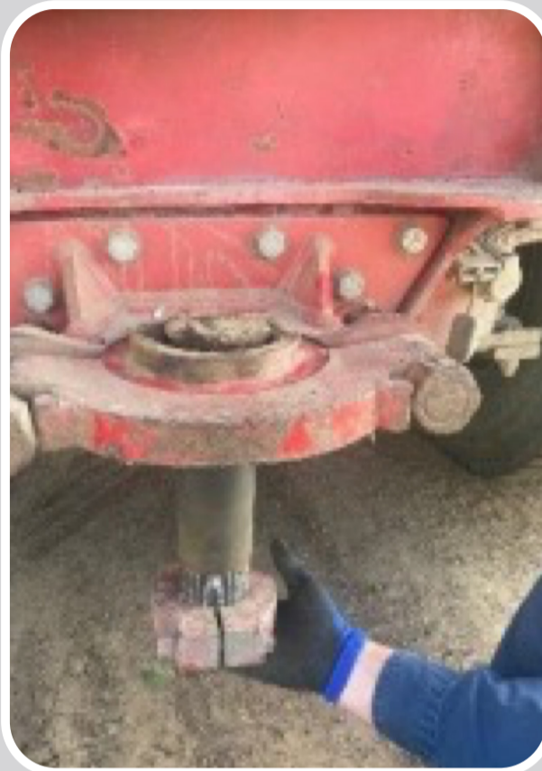
Main nut position on flying saucer hitch assembly.
