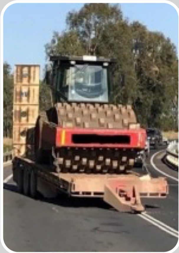
Tri axle tag trailer and padfoot road roller post incident.
