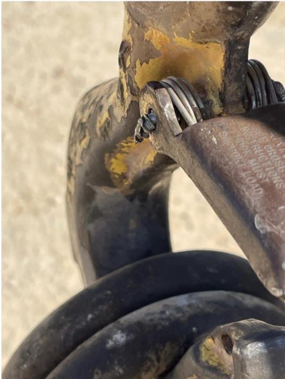
Figure 2: Improvised safety latch
