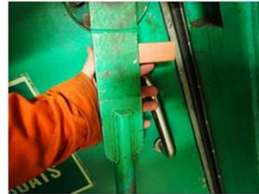
Picture shows the door lock handle swinging free
