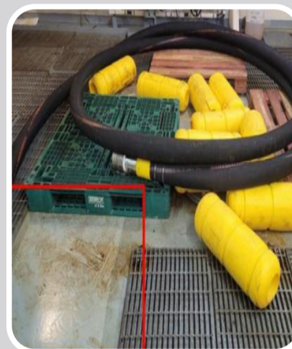
Slippery floor surface contaminated with grease and water from previous activities.
